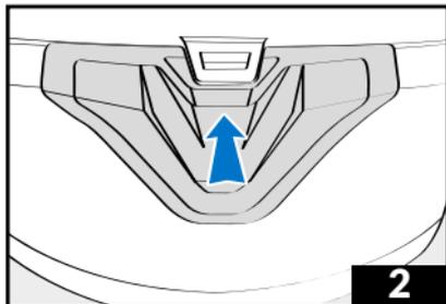
2 - Return the slider to its top position to close the vent.
