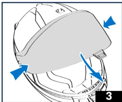
3 - The visor locks into place by pressing on either side of the visor and moving it downwards in a circular motion.
