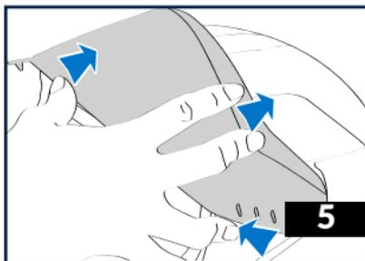
5 - Press the «L» & «R» buttons simultaneously, then use your other fingers on either side to push beneath the visor to remove it towards the back of the helmet. Hold on to the visor at the end of this process.
