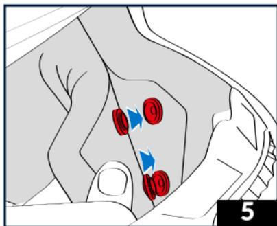
4 & 5 - Turn the helmet over to access the front of each cheek pad and refit each of the three snap fasteners: one at the back and two snap fasteners at the front.
