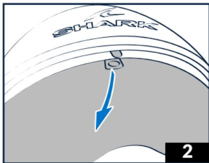
2 - Remove the central fixing pin with a screwdriver or any other pointed instrument.
