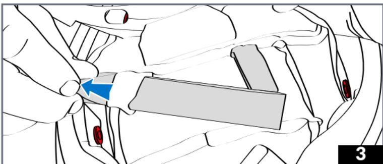
3 - Slide the Morpho Pad through its two securing straps to remove it.
