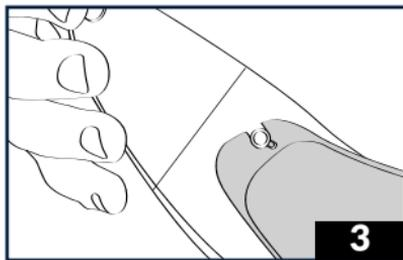
3 - Insert one side of the PINLOCK® lens into one of the two pins at the ends of the visor and hold it in position.
