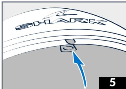
5 - Using a screwdriver or a pointed instrument of any kind, press the central fixing pin from the inside and then re-clip the sun visor by raising it slightly.
