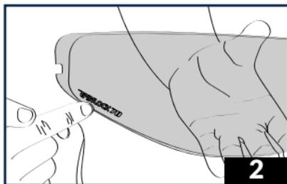
2 - Place the PINLOCK® lens on the visor. The silicone seal of the PINLOCK® lens must be in contact with the inner surface of the visor. The PINLOCK® logo is visible on the outside of the visor.
