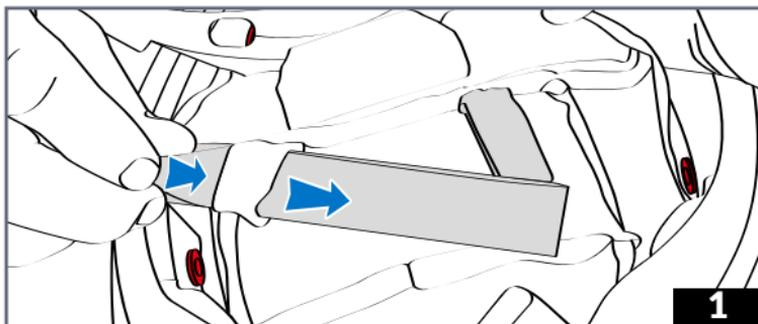
1 - Slide the Morpho Pad through its two securing straps.
