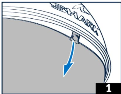
1 - Gently pull the sun visor downwards by hand to visually release its central attachment.
