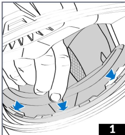
1 - Slide the comfort liner into the helmet. Check that it has been reinserted the right way around. Reposition the front of the comfort liner. Clip the five clips into their slots. Start with the middle clip which must be slid over the arrow shown on the comfort liner support, then one by one the next four side clips.
