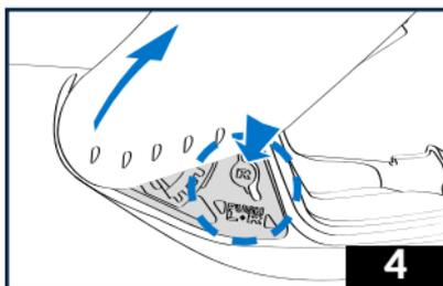
4 - On each of the mechanical side plates, on either side of the visor, locate the button marked «R» on the right side and «L» on the left side.
