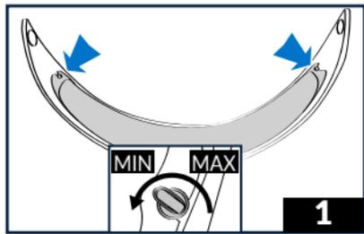
1 - Place the visor on a work surface and on a soft covering. Make sure that the inner surface of the visor is clean. Use a coin to check that the external adjustment levers are positioned inwards (positioned to «INT»).
