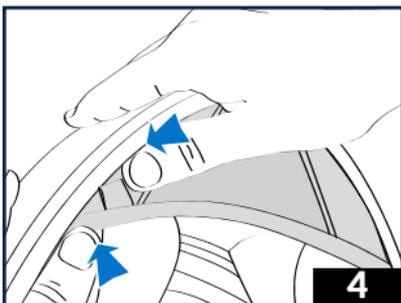
4 - Apply pressure on both sides of the breath guard to ensure that it is firmly secured.
