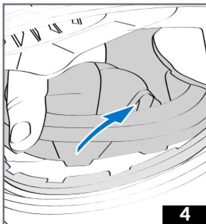
4 - The comfort liner is completely detached and can now be removed.
