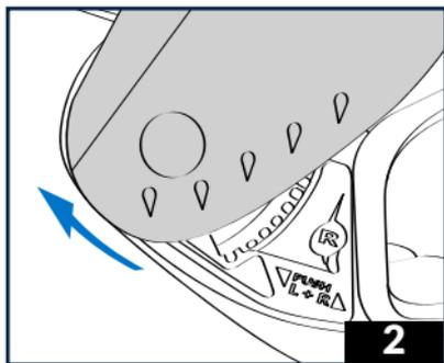
2 - Hold the visor in its raised position in front of the side plates and bring it to rest against the visor step on either side.
