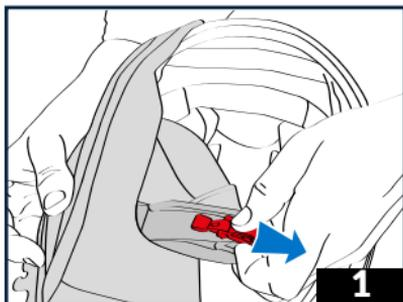
1 - Thread the corresponding chinstrap end through each of the cheek pads. Use the red snap fasteners to guide you in identifying in which direction the cheek pads must be reinserted.
