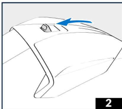
1 & 2 - To use the upper vent, move the button backwards (open) (1); forwards (closed) (2).
