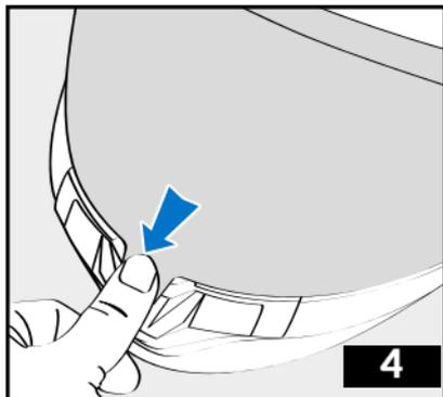
4 - To close the visor completely, lower it by pressing the visor grip on the lock button.
