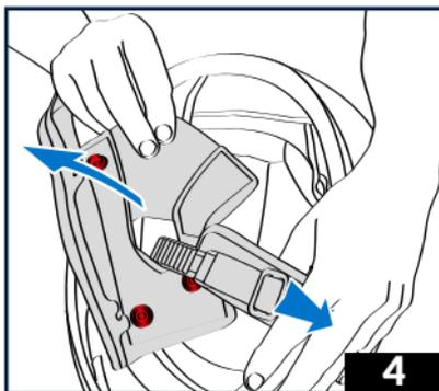
4 - Completely remove each of the cheek pads from the inside by sliding them onto each end of the chinstrap while turning the helmet over if necessary.
