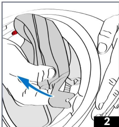
1 & 2 - Slide your hand underneath the back of the comfort liner and pull it towards you on both sides to release the comfort liner from its two clip fasteners.
